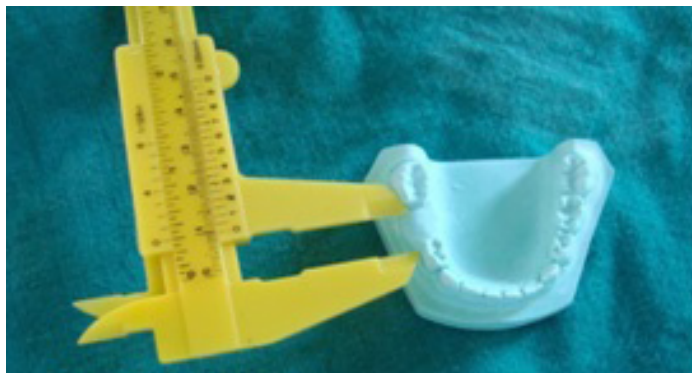
[Table/Fig-5]: Measuring the sample site by vernier caliper
